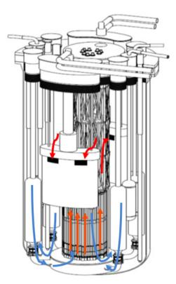
Figure 3-7 Primary Heat Transport System
