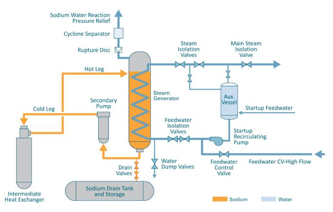
Figure 3-9 Steam Generator and Auxiliaries
