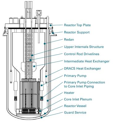
Figure 3-5 ARC-100 3-D Model Reactor Vessel
