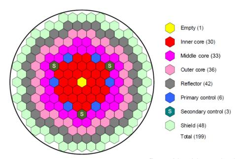
Figure 3-2: Color-coded cross section schematic of the ARC-100 core
