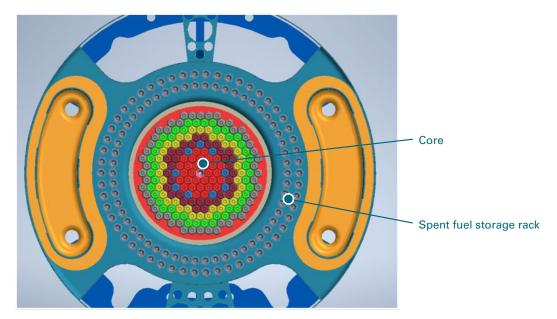
Figure 3-13 Top View of Fuel Storage Schematic
