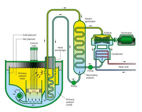
Figure 1-2: Sodium-Cooled Pool-Type Fast Reactor
