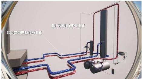
Figure 3-8 Intermediate Heat Transport System
