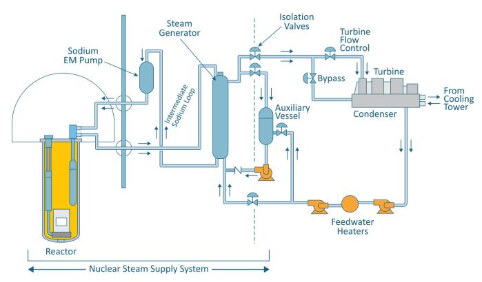
Figure 3-1 ARC-100 Nuclear Systems Schematics
