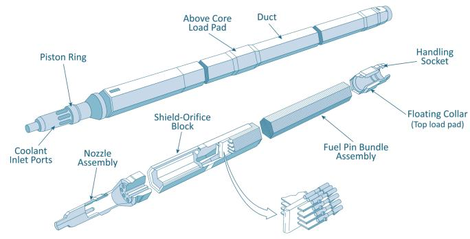
Figure 3-4 Schematic of typical ARC-100 Fuel Assembly
