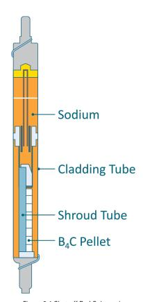
Figure 6-1 Shut-off Rod Schematic
