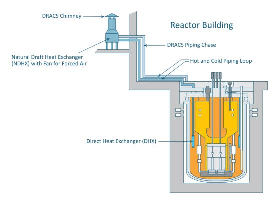
Figure 3-10 Direct Reactor Auxiliary Cooling System (DRACS) schematic
